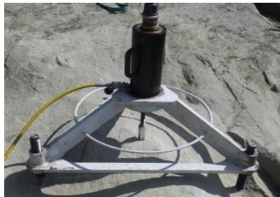
Fig. 2. Own tests on mechanical loosening of rocks within the RODEST project: a) test stand equipment, b) example of a cross-sections through a loosened rock, c) examples of a cross-sections through a loosened rock, specifying the effective anchoring depth H_{ef} , maximum Z_{max} , and minimum Z_{min} loosening range.
