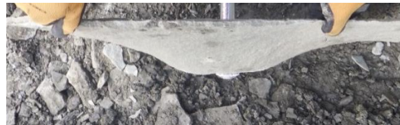
Fig. 2. Own tests on mechanical loosening of rocks within the RODEST project: a) test stand equipment, b) example of a cross-sections through a loosened rock, c) examples of a cross-sections through a loosened rock, specifying the effective anchoring depth H_{ef} , maximum Z_{max} , and minimum Z_{min} loosening range.
